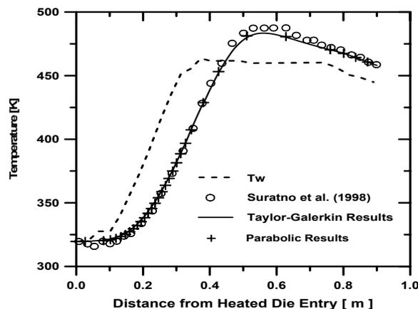
Figure 3a. Results for the axial temperature profile ( $u = 0.1/60$  m·s<sup>-1</sup> and  $FV = 0.7$ )
