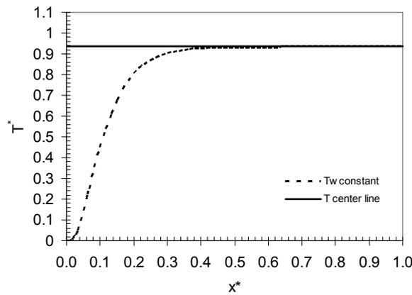
Figure 8 - Predicted center line temperature profiles for the rectangular bar with die-wall set-point temperature constant.
