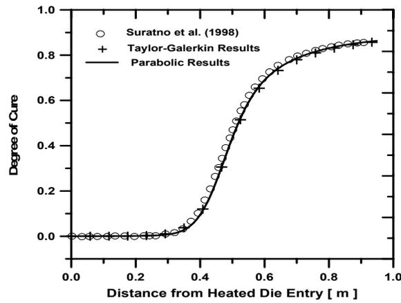
Figure 3b. Results for the axial degree of cure profile ( $u = 0.1/60$  m·s<sup>-1</sup> and  $FV = 0.7$ )
